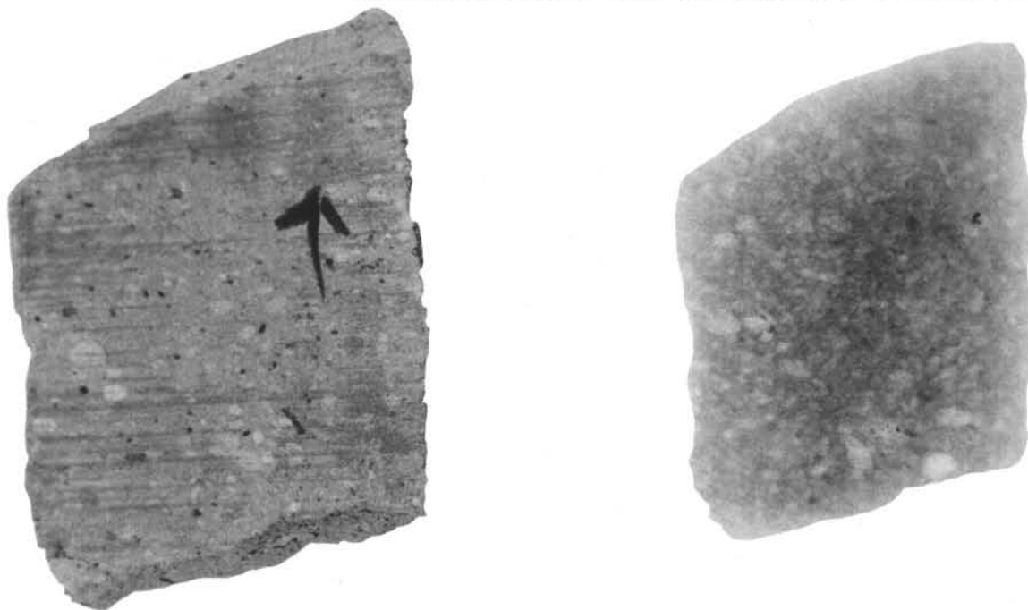
Figure 14. Photograph (left) and radiograph (right) of slice of Sample 290-7-2, 75-81 cm. This nannoplankton-rich volcanic ash is completely homogeneous and displays no sedimentary structures. The larger light-colored parts are larger fragments.
